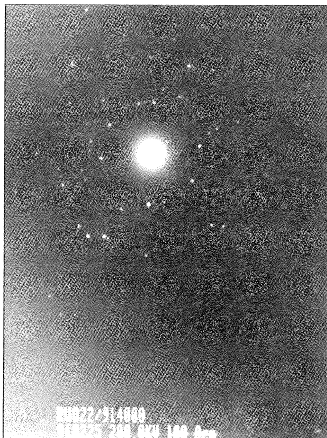
Fig. 9: Electron diffraction pattern from \text{RuO}_2 powder prepared by our method.
