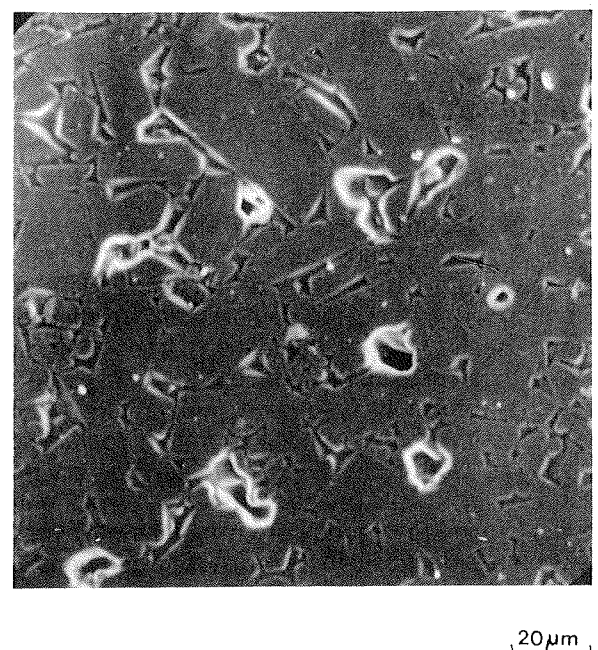
Fig. 2: Microstructure of thermally etched coarse grained alumina a.) Correspondent grain size distribution function.
