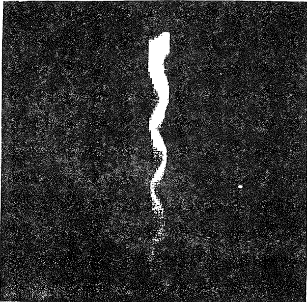
Figure 5: Electrically induced optical waveguide: the signal light beam is traveling along 50 μm wide straight LC waveguide. Since the incidence angle is different from zero but smaller than the one determined by the angle of total reflection, the light beam is reflected back and forth, but stays within the waveguide.
