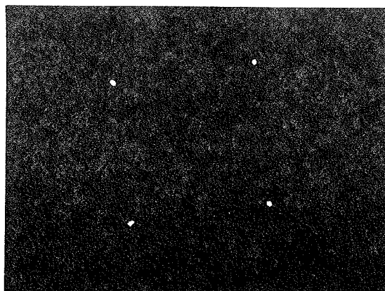
Fig. 6: First order LEED reflexes of a clean iron (100) surface
