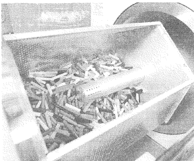
Fig. 4: Treatment of polypropylene pen casings in plasma processor 3000-5D
