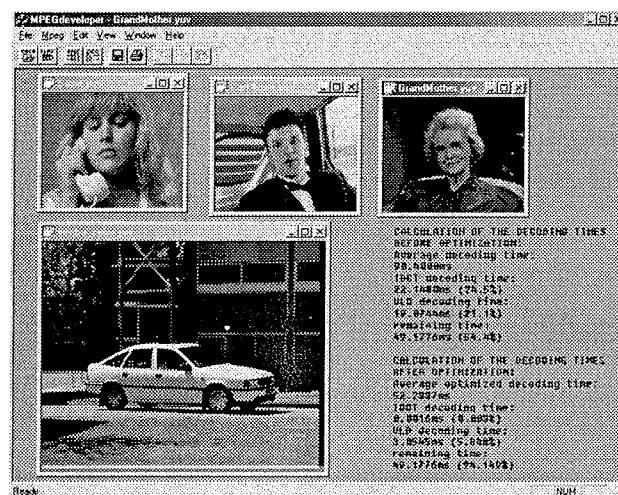
Figure 2: Program for MPEG-2 software simulation
