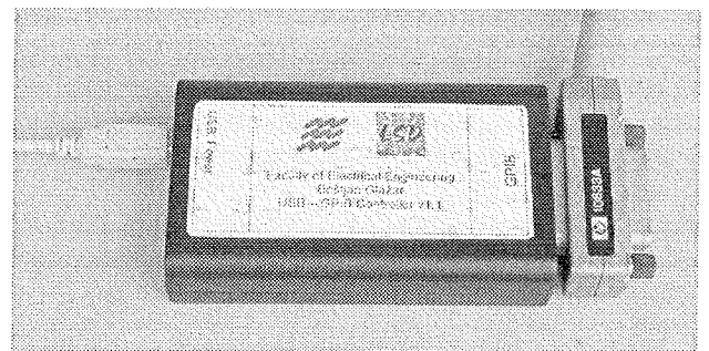
Fig. 3: The controller with connected cables
