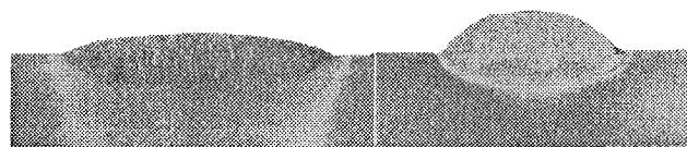
Figure 5: Macrosections of submerged-arc surfacings welded with triple-wire electrode, wires being arranged in the direction transverse to welding direction. Welding parameters: I = 3 \times 195 A, d_0 = 2 mm, L = 28 mm, b = 7 mm, v_w = 30 cm/min, U = 35 V – left, U = 20 V – right.
