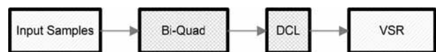
Fig. 5: The extended reference diagram supplemented with the DCL in cascade with the high-pass bi-quad filter.
