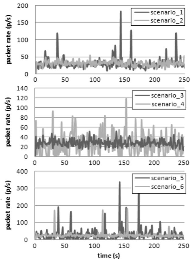
Fig. 6: Modeling measured test traffic 1 in OPNET with six modeling traffics (scenario 1 in 2 with RPG station, scenario 3, 4, 5, 6 with IP station)
