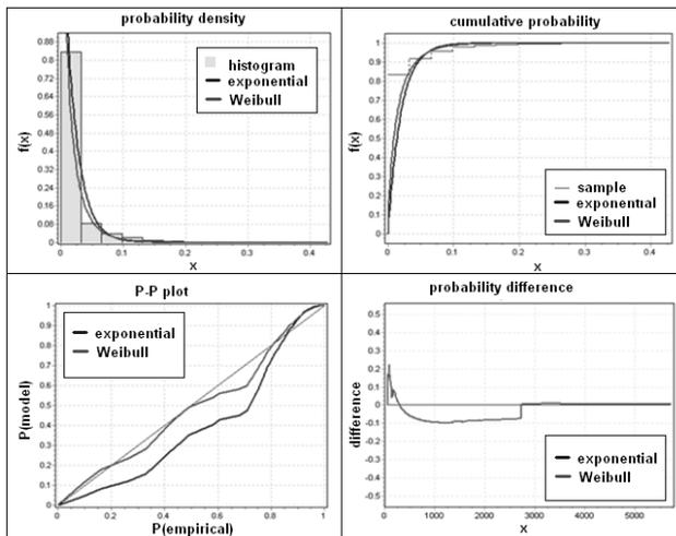
Fig. 2: For the stochastic process of inter-arrival time we chose distribution and estimate parameters of these distributions based on the histogram (upper left), and cumulative distribution function (upper right). Differences between empirical and theoretical distributions in P-P plot (lower left), and deferential distribution (lower right).
