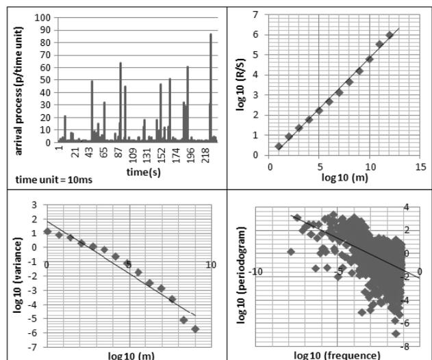
Fig. 1: Estimating parameter H for self similar traffic (upper-left) with the variances method (lower left), R/S method (upper-right) and periodogram method (lower-right)
