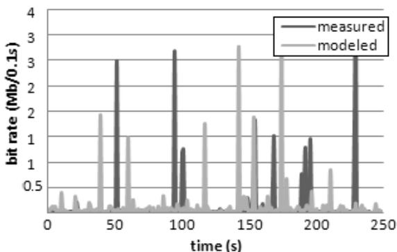
Fig. 8: Comparison between modeling and measuring of test traffic 1 for bit rates.
