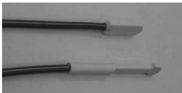
Fig. 10: Example of medical OFS assembly developed by FISO Technologies for skin surface temperature sensing of patient during MRI procedure. The diameter of the blue cables is 3 mm.
