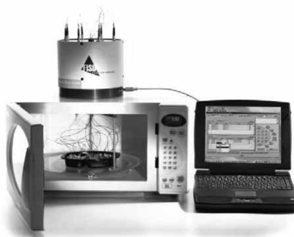
Fig. 9: Commercial kitchen MW oven instrumented by FISO Technologies for multiple point-sensing with F-P temperature sensors.
