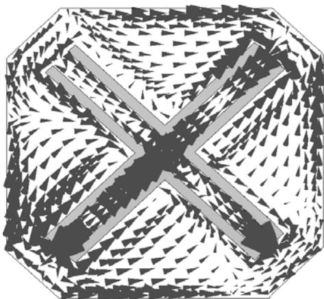
Fig.7: Current distribution on the patch surface at 12.2 GHz.
