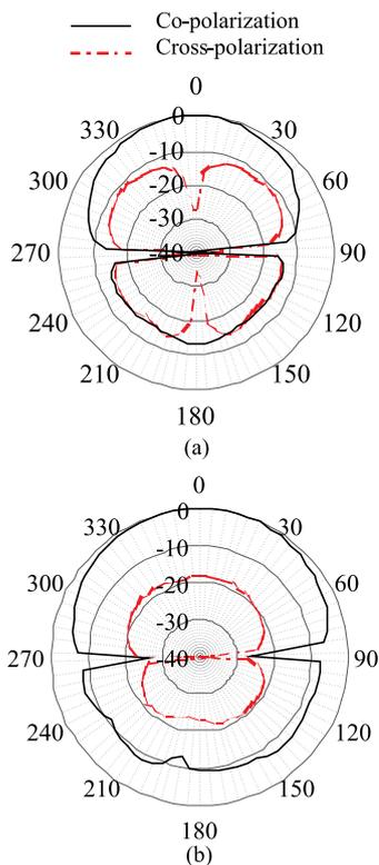
Fig.6: Radiation pattern of the proposed antenna at 12.2 GHz (a) E-plane (b) H-plane.
