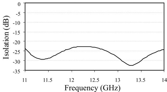
Fig.3: Port isolation of the proposed antenna
