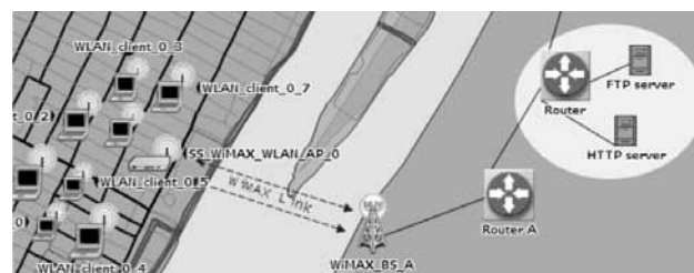
Fig. 1. A WiMax network example with a base station, a core network, and WiMax receivers.
