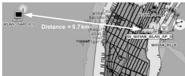
Fig. 8. A long distance (9.7km) between the WiMax access point and the WiMax client.
