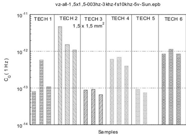
**Figure 8:** Noise quality indicator  $C_Q$  calculated for resistors 1.5 x 1.5 mm<sup>2</sup> for different technologies.
