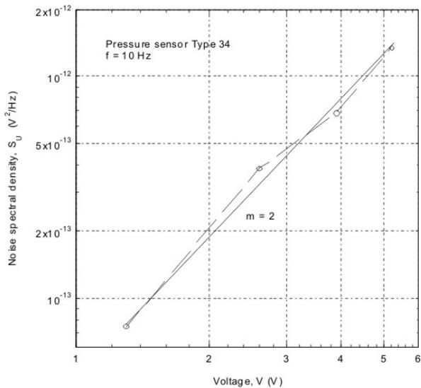
**Figure 6:** Output voltage noise spectral density vs. applied voltage for the pressure sensor Type 2.
