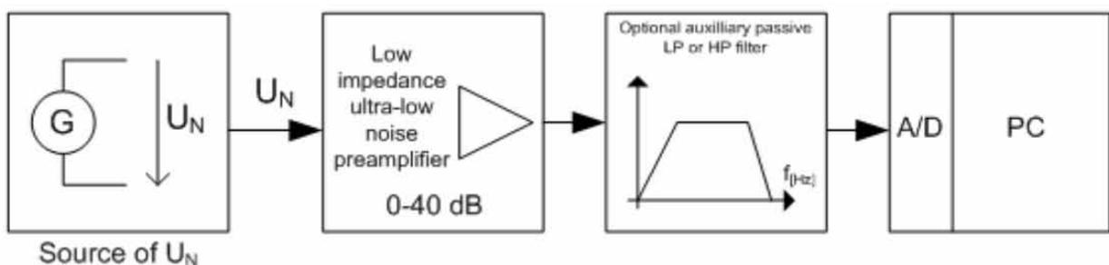
**Figure 4:** Block diagram of the noise experimental set-up.
