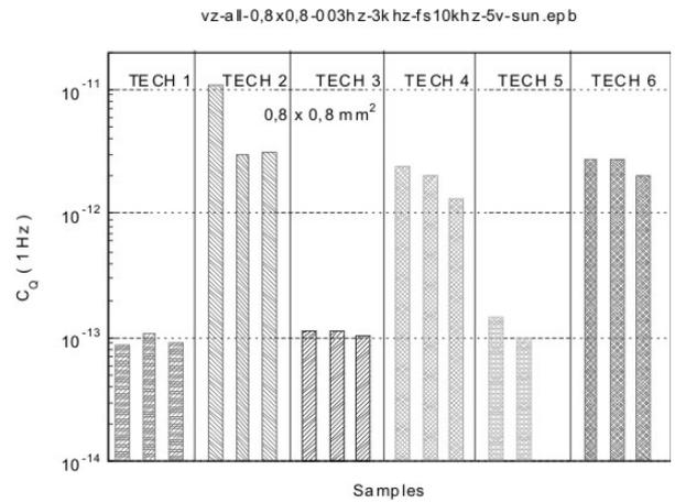
**Figure 7:** Noise quality indicator  $C_Q$  calculated for resistors 0.8 x 0.8 mm<sup>2</sup> for different technologies.
