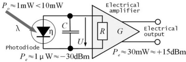
**Figure 5:** Photo-diode receiver.
