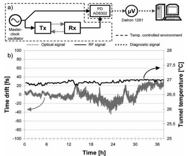
**Figure 10:** a) Long-term stability measurement setup. b) Measured long-term drift at 3 GHz of a 2-fibre system in the accelerator tunnel.
