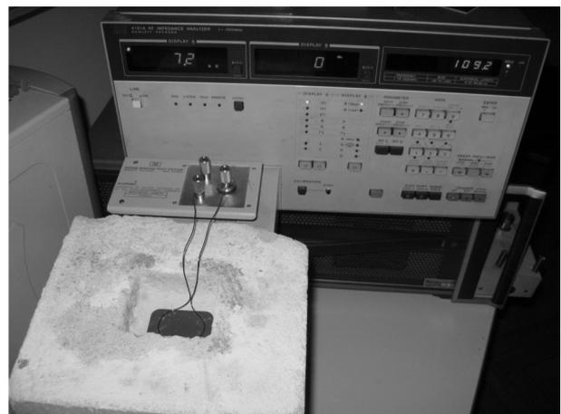
**Figure 19:** Experimental setup for measuring the resonant frequency of the sensor embedded into building material.
