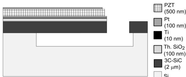
**Figure 3:** Schematic side view of the fabricated device.
