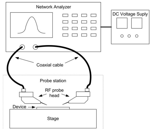
**Figure 4:** Schematic of the measurement setup.
