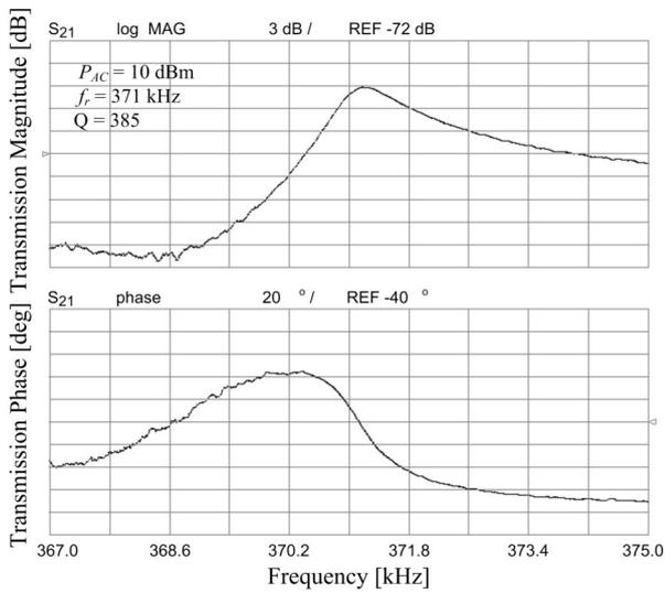
**Figure 5:** Two-port measurements of the transmission frequency response of the 250 μm-long device.
