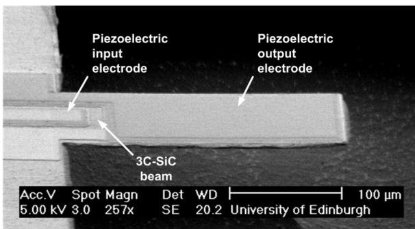
**Figure 1:** Scanning electron micrograph of the fabricated 3C-SiC single-clamped beam (cantilever) resonant device with input and output piezoelectric electrodes placed on the top of the beam.
