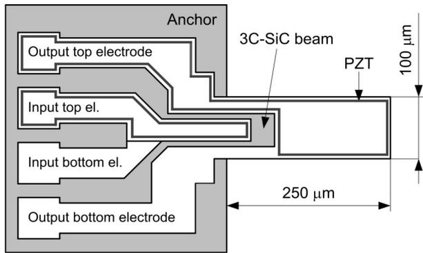
**Figure 2:** Schematic of the designed device with the beam dimensions.
